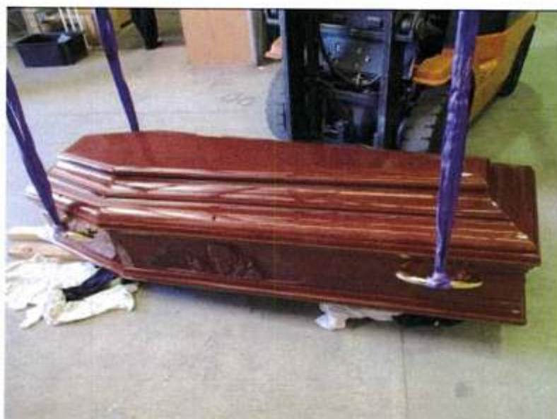
Figure 2: Showing coffin supporting 330kg's.
