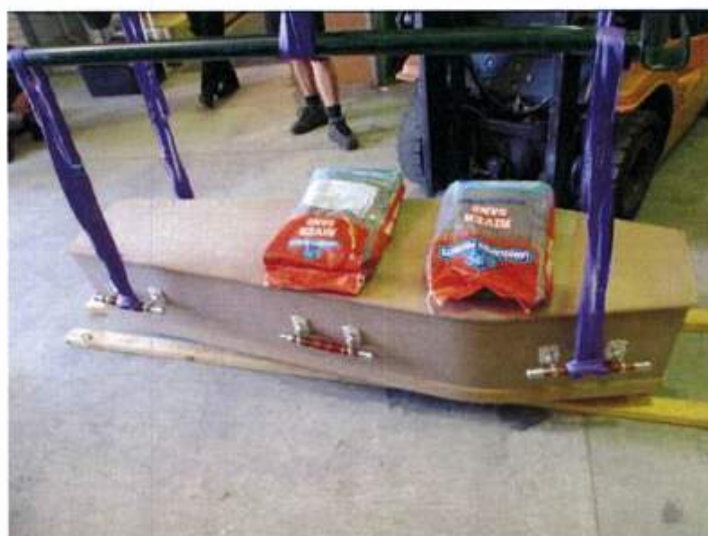
Figure 2: Coffin supporting 323kg's.
